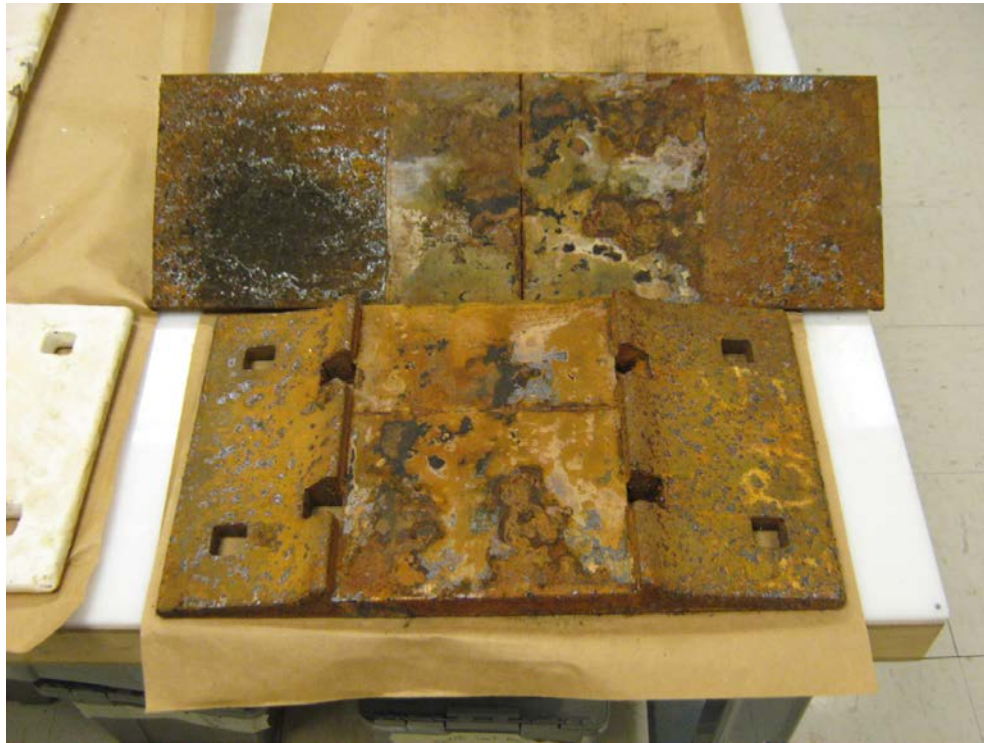
Figure 32. Untreated Samples after 3-Week Exposure
