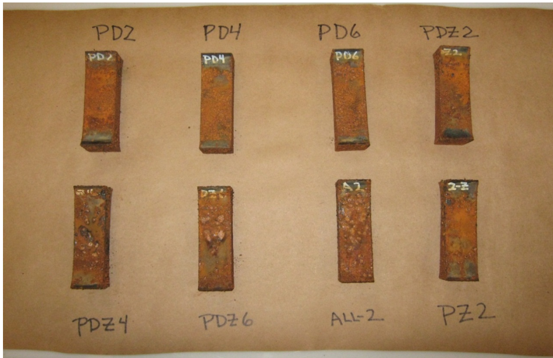
Figure 19. Tops of Samples after 3-Week Corrosion Cycle
