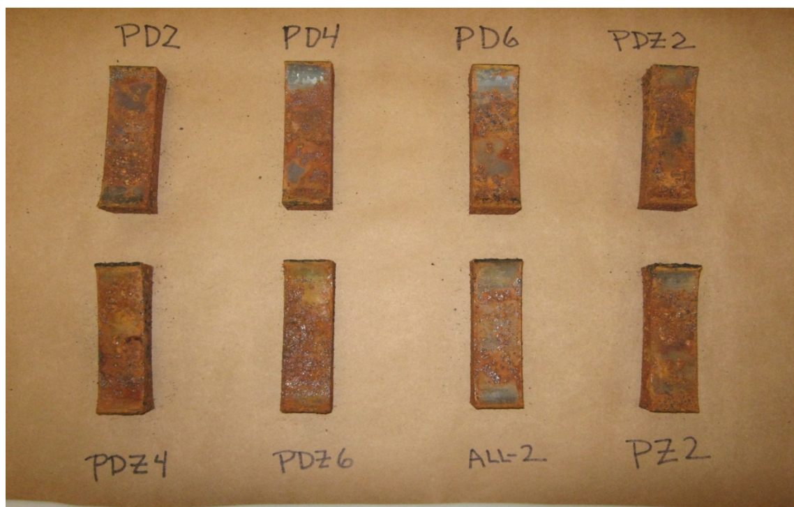
Figure 17. Bottoms of Samples after 3-Week Corrosion Cycle
