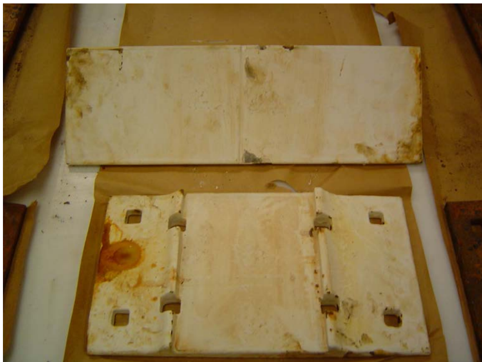
Figure 33. EonCoat® Samples after 3-Week Exposure
