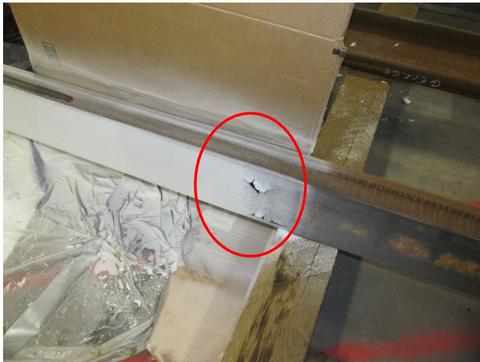
Figure 15. EonCoat® Sprayed Rail Segment
