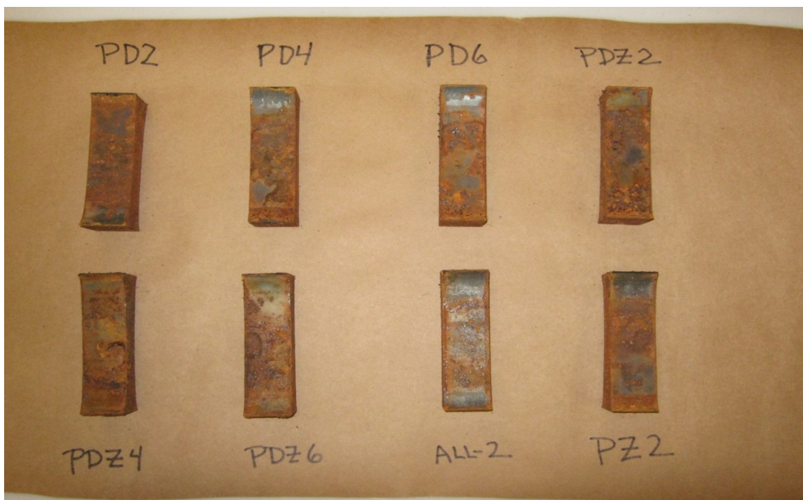
Figure 16. Bottoms of Samples after 2-Week Corrosion Cycle
