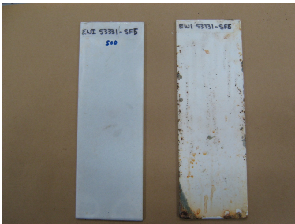
Figure B-5. EonCoat®, Back Side. L→R: 500, 1500 Hours
