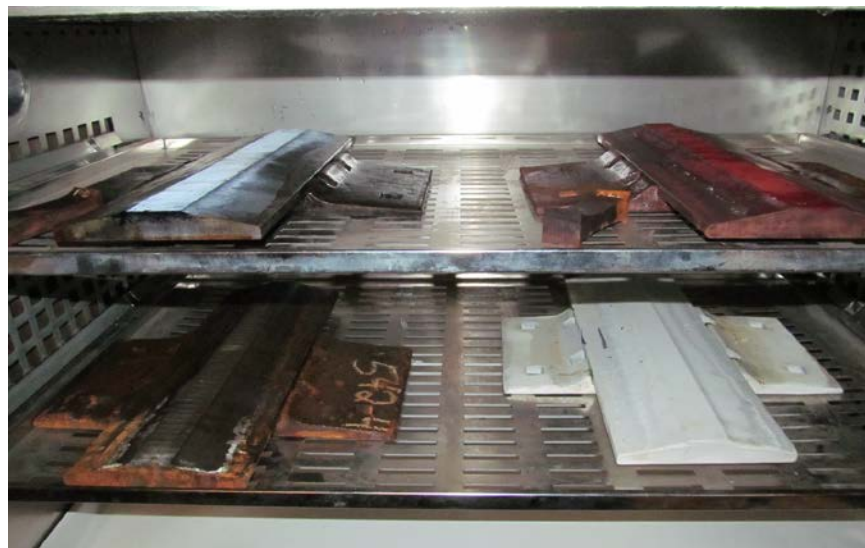
Figure 10. Placement of Samples in Humidity Cabinet
