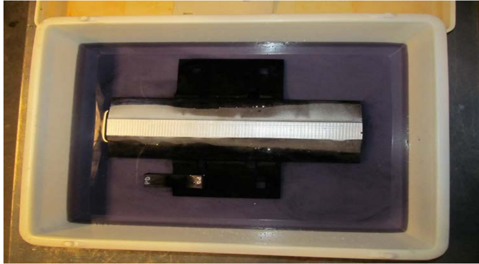
Figure 9. PD Samples on First Exposure to Saltwater
