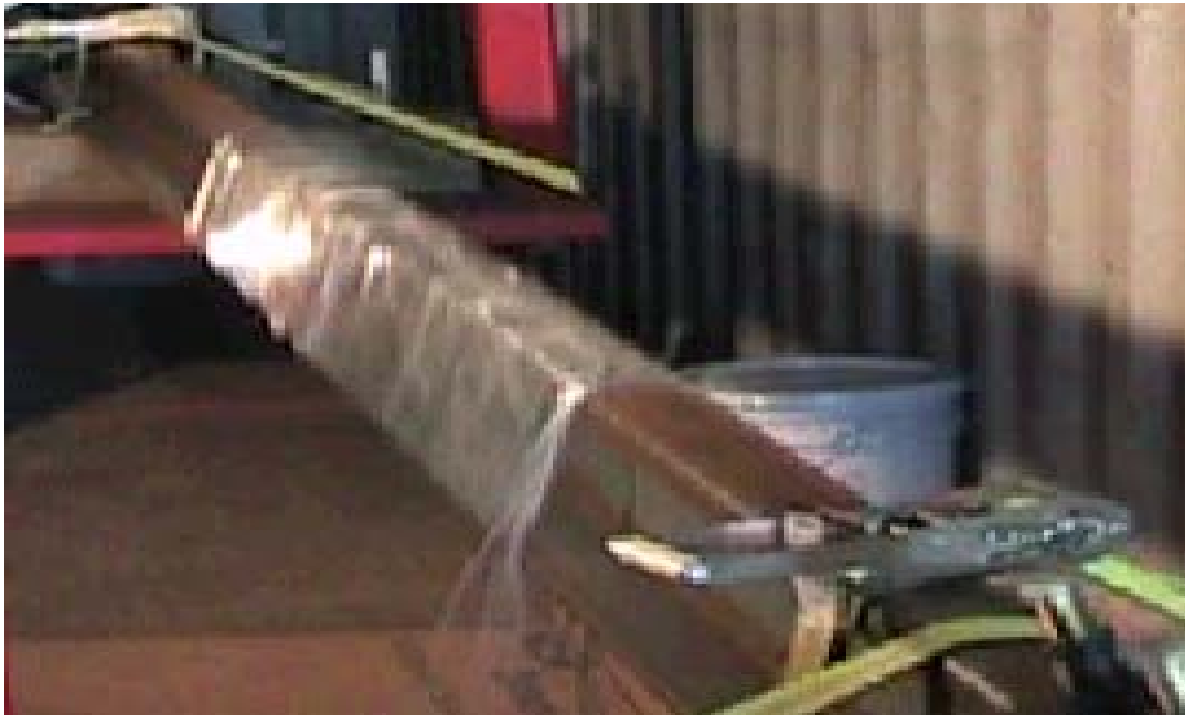
Figure 12. Rail Suspended in Resonant Fatigue Apparatus
