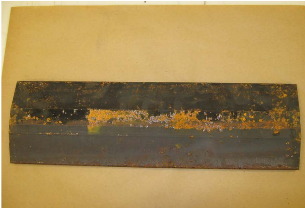
Figure 34. Drip Zone Top Surface after 3 Weeks
